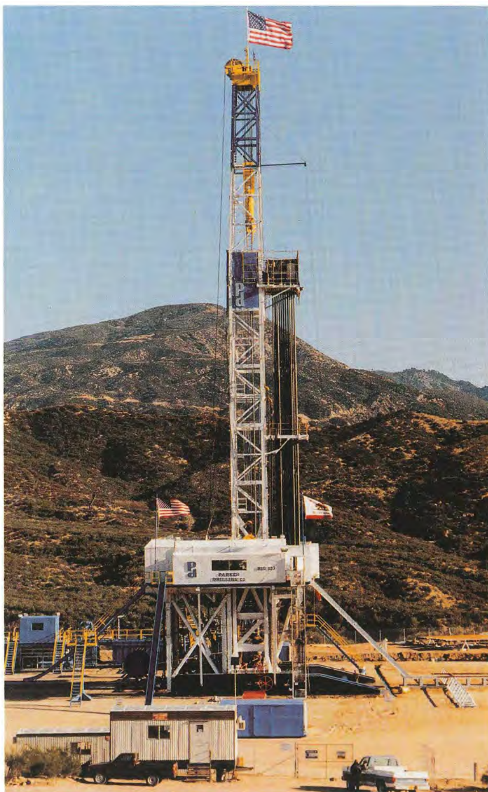
Earthquake research. At Cajon Pass, in the earthquake-prone region of the San Andreas fault in California, scientists have drilled a hole deep enough to sample the earth's crust and monitor the forces that may give early warnings of an earthquake.
