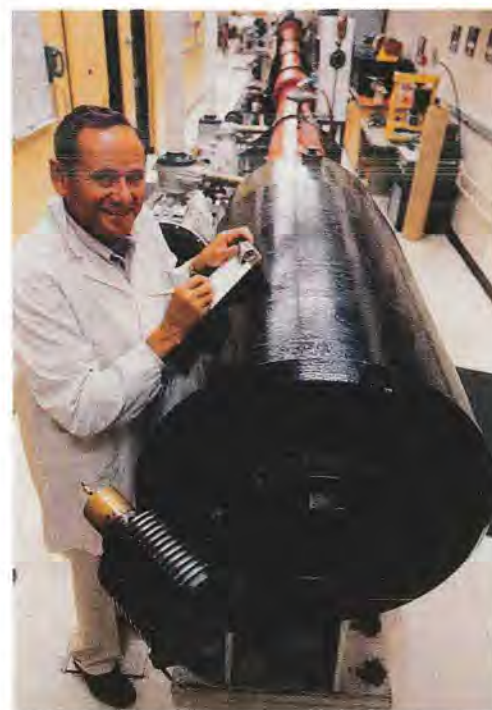
Core of the matter. Thomas J. Ahrens checks procedures for firing Caltech's light gas gun, which simulates the high pressures at the earth's core.
